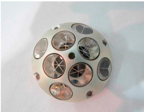
Fig. 3. The Laser Retroreflector Array (LRA). The unit is 50 mm in diameter at the base and 16 mm in height. Photo credit: SpaceIL/Xiaoli Sun/GSFC.
