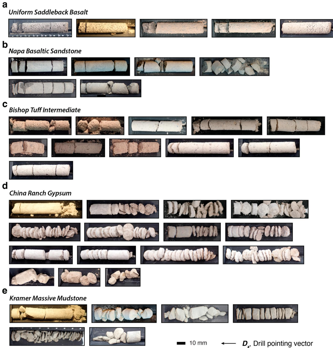
Figure 11. Results of coring attempts with the Mars 2020 Qualification Model Dirty Testing (QMDT) testbed at Jet Propulsion Laboratory (JPL). Shown are five different lithologies in order of decreasing compressive strength. (a) Five samples of the Uniform Saddleback Basalt, a massive aphanitic or very fine-grained to finely ophitic olivine basalt from the Early Miocene Tropic Group collected near Boron, CA (Dibblee Jr, 1958; Moeller et al., 2021; Peters et al., 2008). (b) Six samples of the Napa Basaltic Sandstone, a volcanogenic basaltic sandstone from the Early Cretaceous to Late Jurassic mélange of the Great Valley Sequence collected at the intersection of Capell Valley Road and Monticello Road in Napa, CA (Delattre & Sowers, 2006; Moeller et al., 2021). (c) Eleven samples of the Bishop Tuff Intermediate, a hypocrySTALLINE rhyolitic pyroclastic rock from the Pleistocene Bishop Tuff, collected in northern Owens Valley, CA (Moeller et al., 2021; Wilson & Hildreth, 1997). (d) Fifteen samples of China Ranch Gypsum, a hydrated sulfate with massive, layered and vein occurrences from the Tertiary China Ranch Beds collected along China Ranch Road near Tecopa, CA (Hillhouse, 1987; Moeller et al., 2021). (e) Six samples of the Kramer Massive Mudstone, a sandy-silty clay provided by U.S. Borax, Kern County, CA (Moeller et al., 2021; Siefke, 1991).
